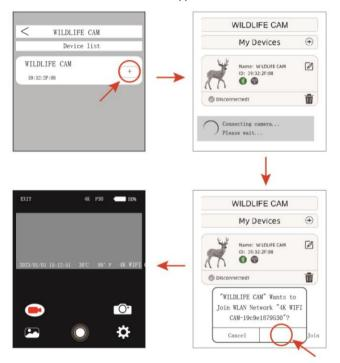
As shown above, when the Wi-Fi icon turns green this means the app has connected with your mobile device. The mobile device will then show the real-time preview screen.
